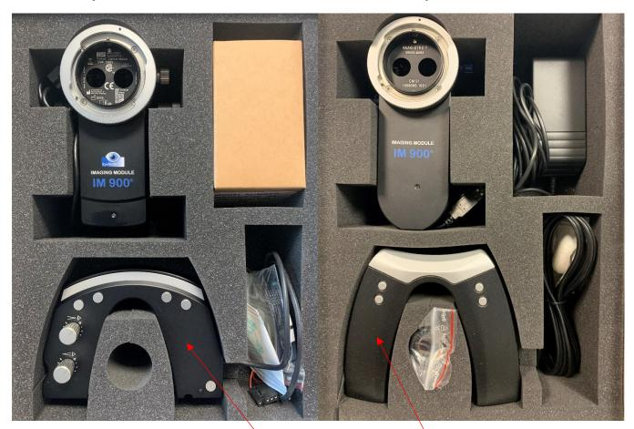
Current IM system (900 or 600) for LED slit lamps BQ900 and BP900. Use USB3 Port to connect trigger (RM02) to computer.
