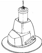
**Removing Covers:** The back cover is held on by one screw. The main cover is held on by three screws located under the base casting. To remove cover:
