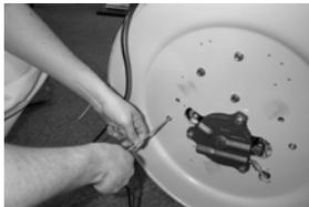
5. Using a thin blade screw driver, starting at the top of cover, gently pry the two halves apart until the cover is separate.
