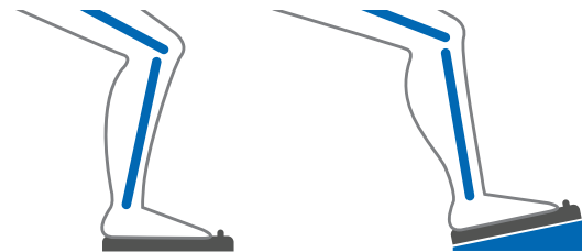
Elevated, angled surgical foot pedals allow for a more natural position for the leg.
